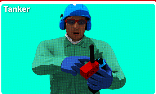
Emergency shutdown from tanker
