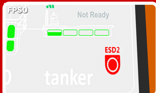
ESD feedback signal in control room
